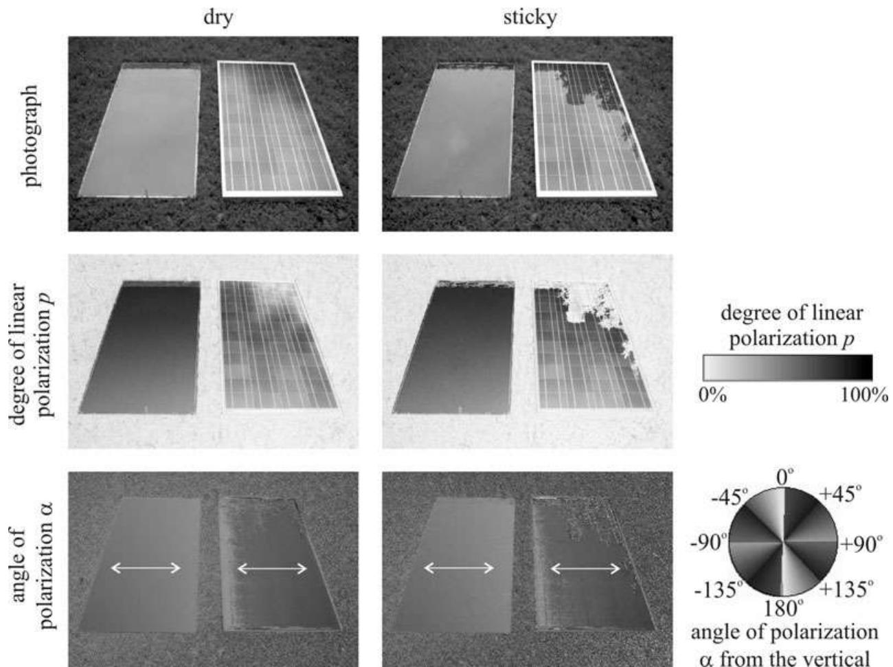
**Figure 2.** Photographs and reflection-polarization patterns of the two horizontal (dry and sticky) solar panels used in the choice experiments with mayflies, caddis flies, dolichopodids, and tabanids. Double-headed arrows show the direction of polarization of reflected light. The polarimeter viewed toward the antisolar meridian and the angle of elevation of its optical axis was  $-35^\circ$  from the horizontal.
